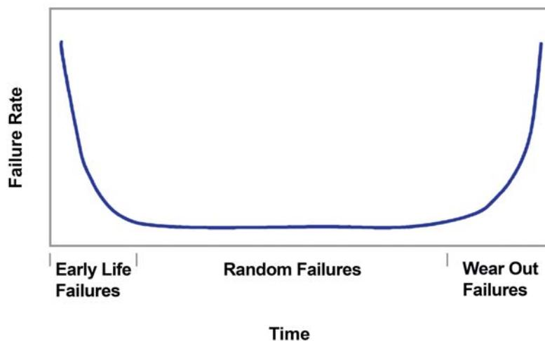
Figure 5: Bathtub curve showing probability of failures over the technical lifetime of a product or project [21]
