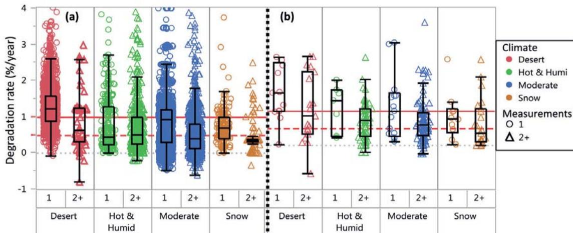
Figure 4: Degradation rate for x-Si PV module depending on climate (Jordan 2016)
